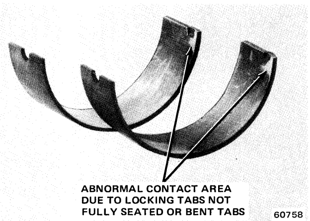
Fig. 1B-36 Locking Tab Inspection
